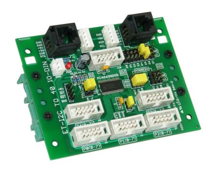
ET-I2C TO 40 IO-DIN is I/O EXPANSION BOARD for 40-BIT MCU that is divided into 8-BIT 5-PORT and it is I2C BUS Interface. Specifications of this board are listed as follows;
